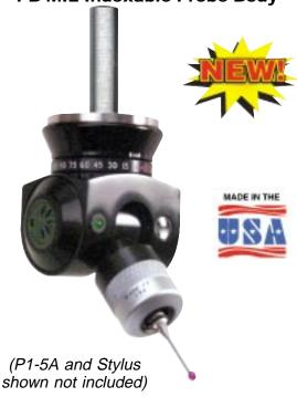
The PB-MIL is a manually indexable probe body that allows 168 probe positions and eliminates the need to requalify the probe styli. It can be used with our P1-5A touch trigger probe, or any M8 threaded touch trigger probe. Colored increments and a magnifying window clearly indicate current probe position.
