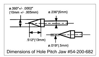
**▲**#54-200-682-The Max-Cal Multi-Purpose Caliper measures center-tocenter distance between bores under .39" (10mm). The adjustable outside jaw permits measuring of even as well as uneven planes.
