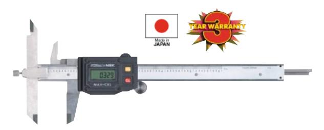
The Max-Cal Offset Caliper measures dimensions on uneven or offset planes easily and accurately. The long (4"/100mm) adjustable outside jaw permits access to a large range of uneven surfaces for a wide variety of measuring applications.
