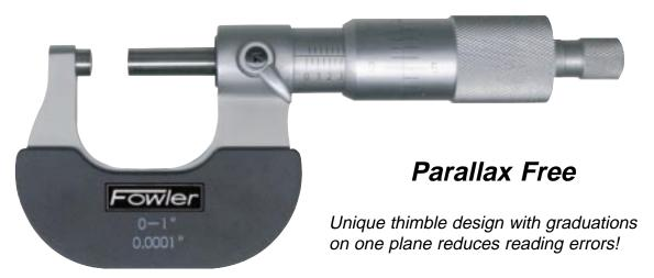
Quick reading micrometer with a special parallax free spindle and sleeve. Easier to read than standard vernier micrometers, the barrel is graduated in 0.001" with a tenth reading vernier.
