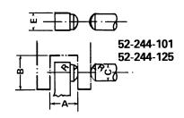
The back side of the anvil stem of Fowler Ball-Anvil Tube Micrometers is cut away, making it slim enough to insert into small parts such as sleeves, collars, tubing and other cylindrical workpieces to measure wall thickness.
