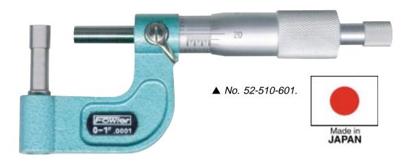
**Fowler Rod-Anvil Tube Micrometers** are positioned at a 90° angle in respect to the axis of the spindle, making it practical and convenient for measuring wall thickness of tubings and other workpieces with cylindrical walls.
