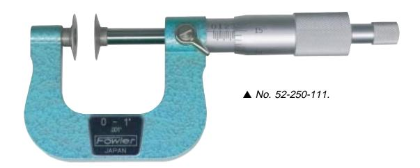
**Fowler Disc Micrometers simplify** measuring thickness of difficult, closely spaced sections, ribs, keys, fins, cutting edges on forming tools, chordal thickness of gear teeth and more. The extra large diameter disc will enter normally inaccessible places such as narrow grooves, slots and recesses.
