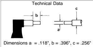
Fowler's Digital Spline Micrometers offer you the convenience of a digital counter for measuring recesses, splines and grooves of forming tools.
