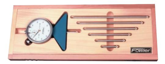
Fowler's Dial Depth Gage comes with six interchangeable rods with a 0—22" capacity. Provides rapid direct reading measurement of hole depths.
