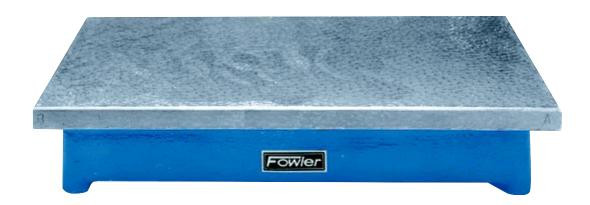
Cast Iron Surface Plates are made from close-grained cast iron, heat treated and stress relieved to a hardness of 170—220 BHN.
