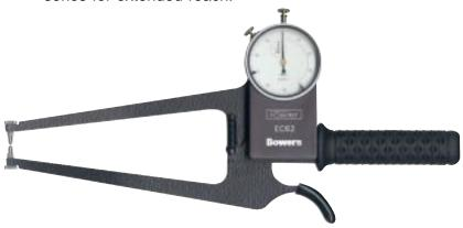
▲ External Dial Calipers #52-554-600 and 900 series are for use where access is limited.
