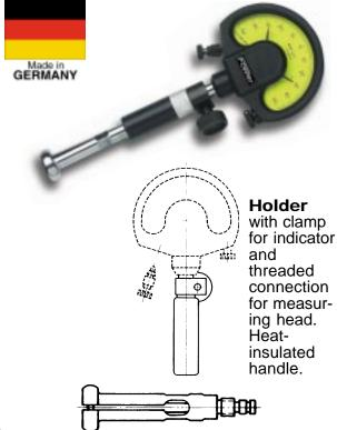
Measuring head consists of interchangeable measuring probe and expander pin. Probe spring-loaded and of split design. Individual measuring heads available on request.
