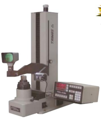
▲ # 54-188-745 Presetters currently equipped with Metronics' Tool-Chek readout. Indicator holder not included with Presetter.
