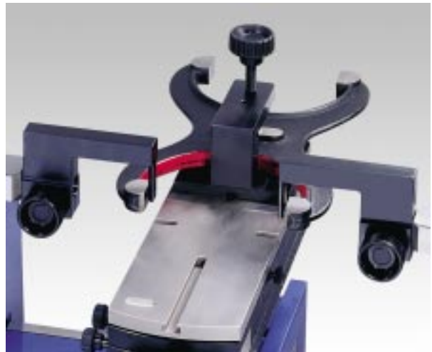
▶ Checking of snap gages from .473 to 6" (12 to 150mm) using #54-196-160, 54-190-815 and 54-197-162
