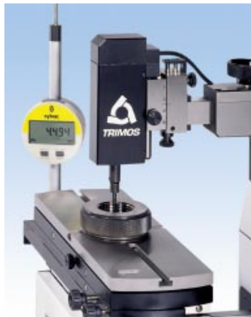
▲ checking of threaded ring gages from pitch 0.7 to 6mm/48 to 4 threads per inch (max. internal dia. 7.08"/180mm) using 54-197-011, 54-197-142, 54-197-074 & 54-197-075
