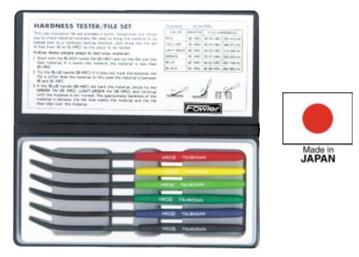
Fowler's Hardness Tester File Set is an inexpensive, easy-to-use method for determining material hardness by sliding the file across the object's surface. Six color coded files indicate hardness from 40 to 65 HRC. Conveniently packaged in a leather-like case with a velcro lined flap, the files are approximately .157" in diameter and 7" in length (4.3Ø x 175mm).
