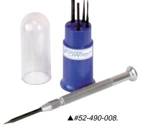
Jewelers' miniature screwdrivers feature a finger support swiveling head that can be held and rotated for precise control while removing and tightening screws.
