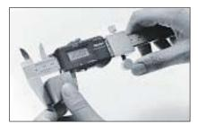
Push the whole sliding unit against your masterpiece. (Gage Block used here) Lock with clamp.
