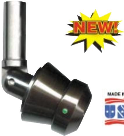
Providing a sturdy mount for our P1-5A or any M8 touch trigger probe, the PB-1 features three LED's spaced 120° apart which allow trigger hits to be easily assessed from any angle. The shank can also be swiveled 180° to allow for easy positioning. The PB1 will also accept any length M8 threaded probe extensions.
