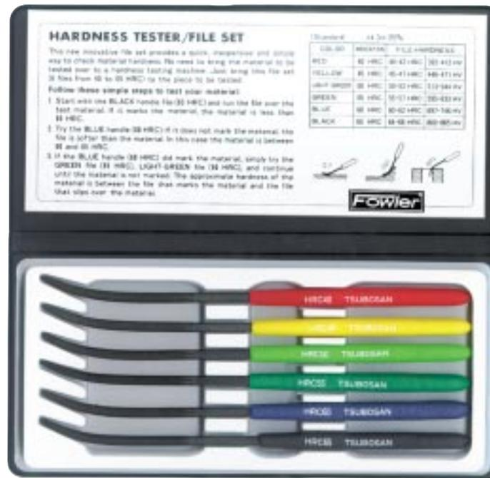
Fowler's Hardness Tester File Set is an inexpensive, easy-to-use method for determining material hardness by sliding the file across the object's surface. Six color coded files indicate hardness from 40 to 65 HRC. Conveniently packaged in a leather-like case with a velcro lined flap, the files are approximately .157" in diameter and 7" in length (4.3Ø x 175mm).
