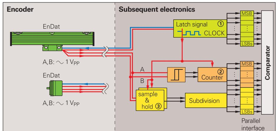
The code value transmitted over the serial interface unambiguously identifies one incremental signal period. The position value is absolute within one sinusoidal period of the incremental signal. The subdivided incremental signal can therefore be appended in the subsequent electronics to the serially transmitted code value.
