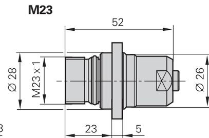
**Flange socket:** Permanently mounted on the encoder or a housing, with external thread (like the coupling), and available with male or female contacts.
