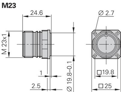
**Right-angle flange socket (rotatable)** on adapter cable inside the motor with connection for temperature sensor
