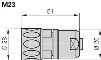
**Coupling insulated:** Connecting element with external thread; Available with male or female contacts.
