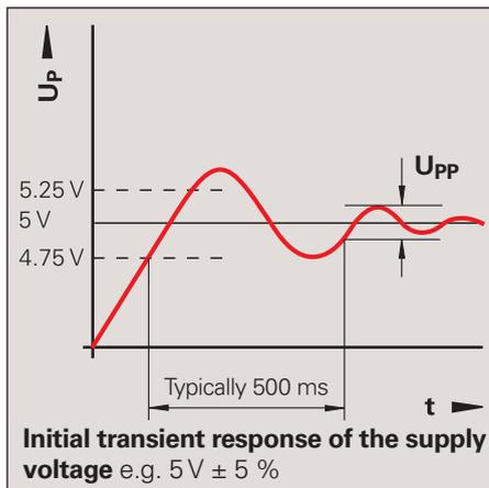
The values apply as measured at the encoder, i.e., without cable influences. The voltage can be monitored and adjusted with the device's **sensor lines**. If a controllable power supply is not available, the voltage drop can be halved by switching the sensor lines parallel to the corresponding power lines.
