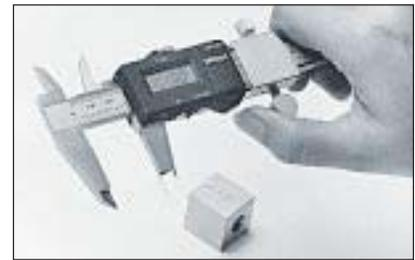
3. Open and close jaws with snap lever to check workpieces allows .079"(2mm) retraction.
