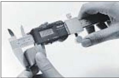
1. Push the whole sliding unit against your masterpiece. (Gage Block used here) Lock with clamp.
