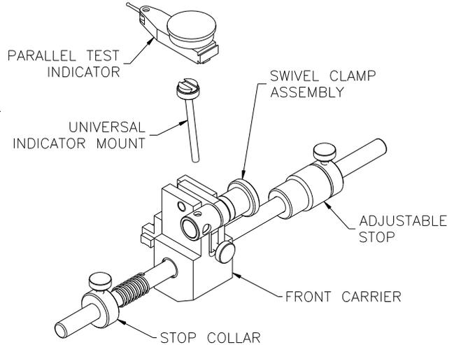
Figure 7. Front Carrier Assembly
