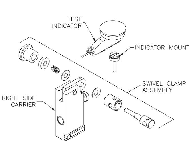
Figure 6. Right Side Carrier Assembly
