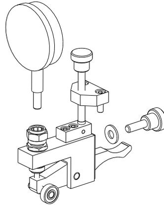
Figure 11. Roller Checking Attachment with Fine Adjust
