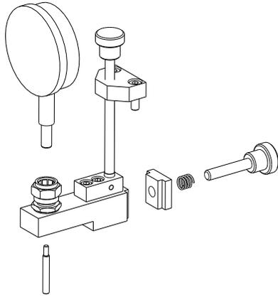
Figure 10. Dial Indicator Holder With Fine Adjust
