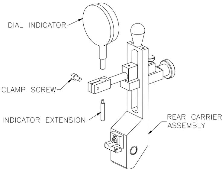
Figure 8. Rear Vertical Carrier with Dial Indicator
